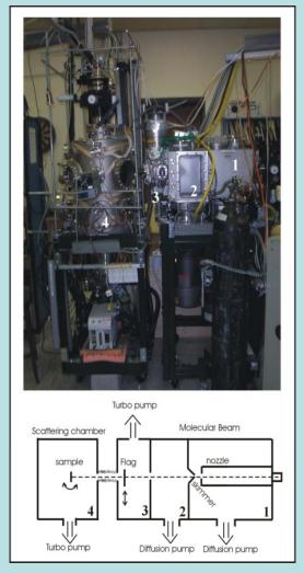
Adsorption/reaction dynamics: The workhorse of our group is this molecular beam scattering system, it's a kind of LASER but we use beams of "real" particles (He, alkanes, water, alcohols, CO, NO, CO<sub>2</sub>, etc..). We just could upgrade the system by an XPS spectrometer and larger pumps (DoE).
