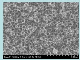
The main application for this fancy carpet is photo catalysis including solar cells, water splitting, etc.. Here we work together with P. Schmuki's group (Germany).
