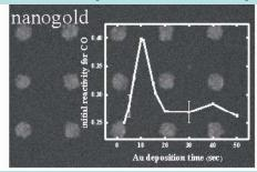
Model nano array catalysts consist of a predetermined structure of nanometal dots with perfect control over their morphology which is pertinent for model studies. This project is a collaboration with national labs in Berkeley and Argonne/Chicago. Electron beam lithography is used to manufacture the samples.
